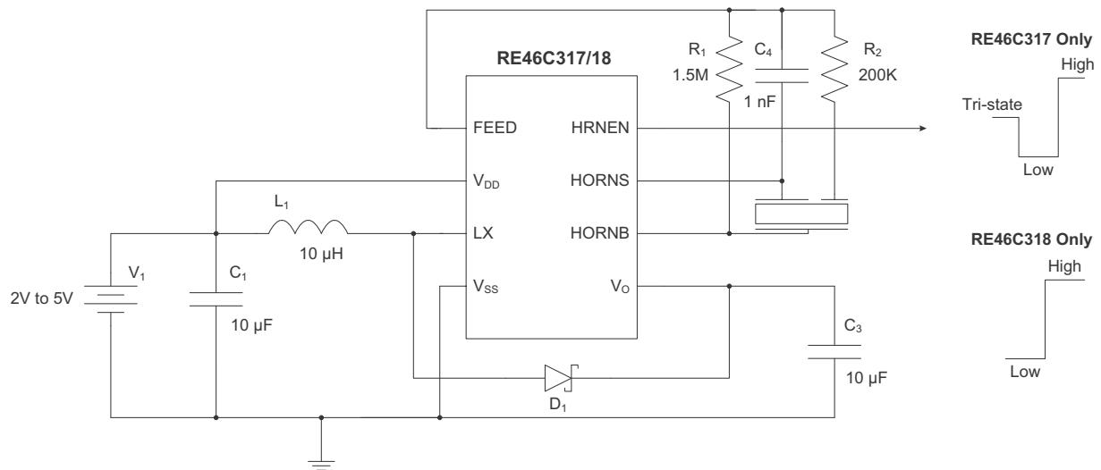
**Note 1:** Schottky diode D<sub>1</sub> must have the maximum peak current rating of at least 1A. For best results, the forward voltage spec should be less than 0.5V at 1A.
