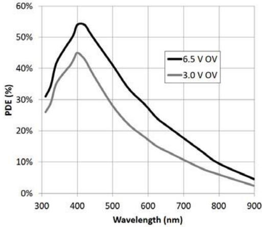
**Figure 5: PDE at Peak  $\lambda$  vs. OV**
