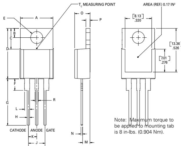
Note: Maximum torque to be applied to mounting tab is 8 in-lbs. (0.904 Nm).
