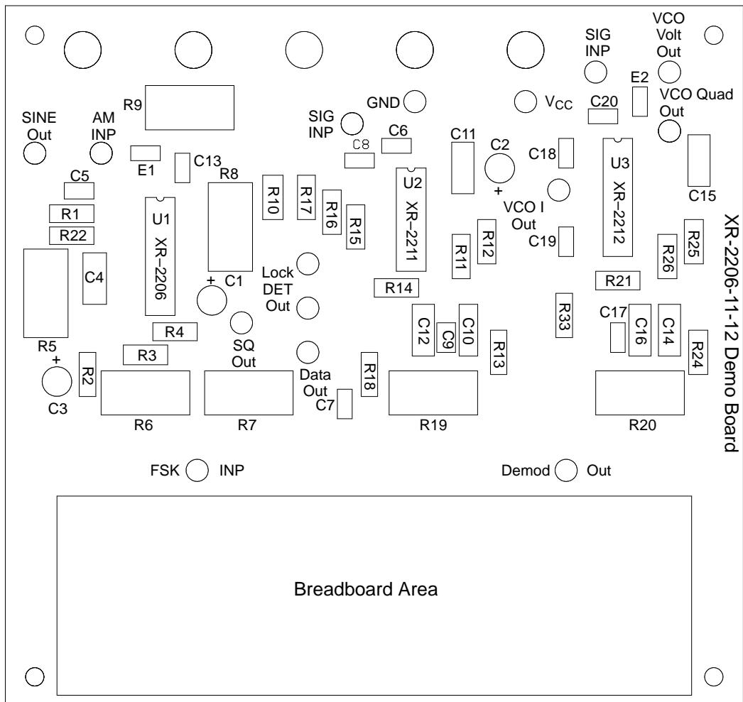
Figure 1. Demo Board Component Layout
