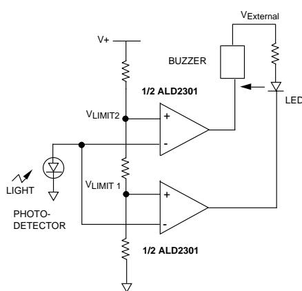
LED turns on as photo-detector voltage reaches  $V_{LIMIT1}$ . Both LED and horn turns on as photo-detector voltage reaches  $V_{LIMIT2}$ .
