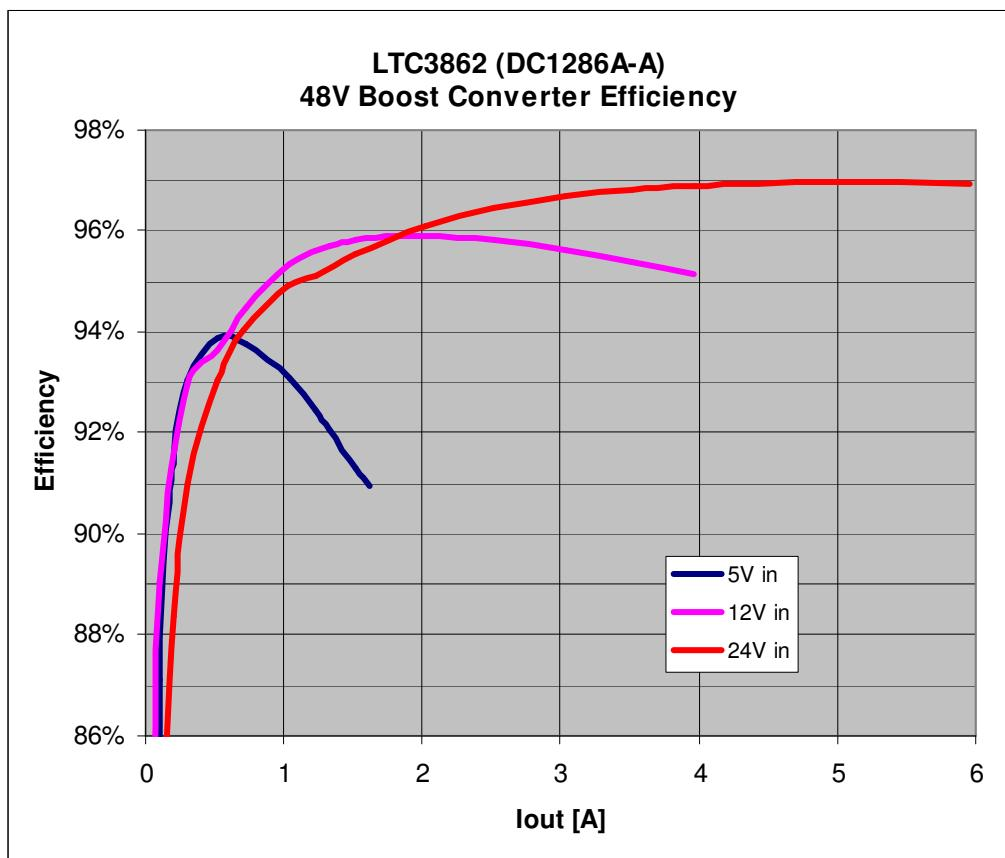
Figure 3. DC1286A-A Efficiency
