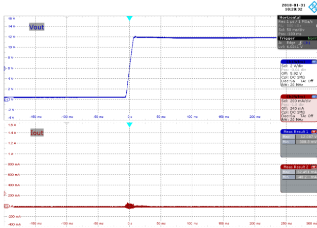
Figure 56 – 90 VAC 60 Hz, No-Load Start-up. Upper: V_{OUT} , 2 V / div., 50 ms / div. Lower: I_{OUT} , 200 mA / div., 50 ms / div.
