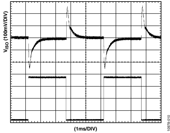
Figure 10. Typical Transient Load Response, 5 V Input, 3.3 V Output, 10% to 90% Load Step
