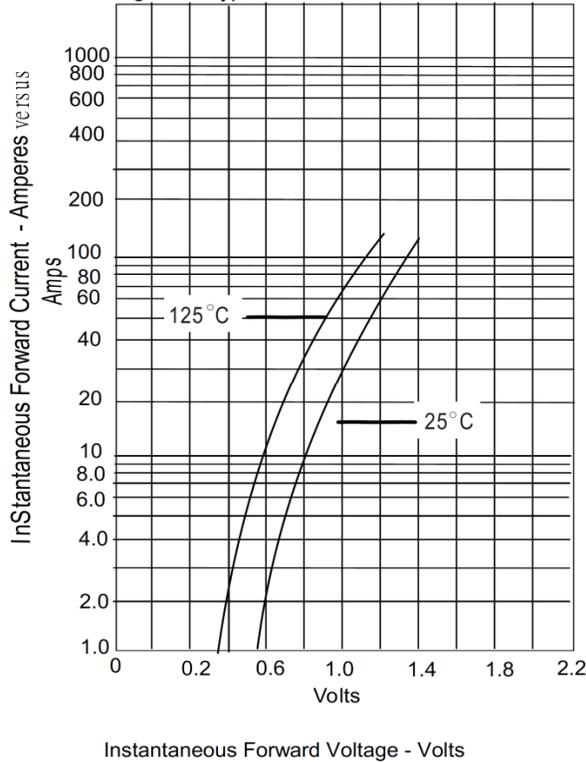
Figure .2-Forward Derating Curve
