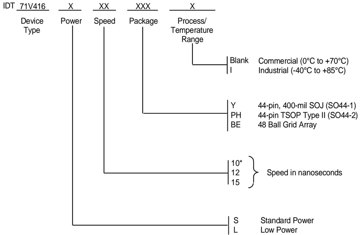
\* Commercial only for low power 10ns (L10) speed grade and Industrial only for standard power 10ns (S10) speed grade.
