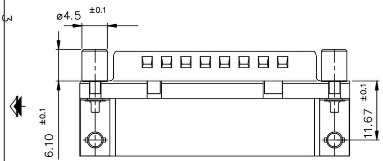
PC card drilling dimensions(after plating)
