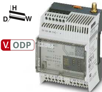
Communication via ODP protocol, 2 additional analog inputs
