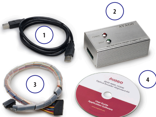
Figure 2. Alignment kit components for HEDS-8949
