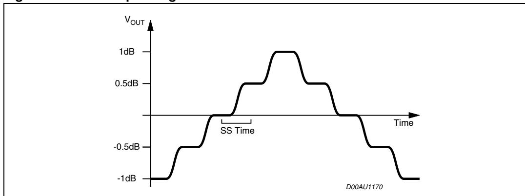
1. For steps more than 0.5dB the Soft-step mode should be deactivated because it could generate a hard 1dB step during the blend-time.
