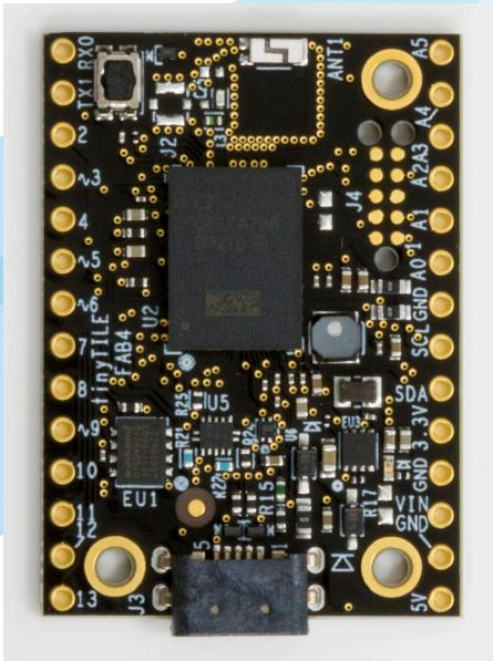
tinyTILE is a miniaturised adaptation of the Arduino/Genuino 101 board, measuring approx 35 x 26mm.
