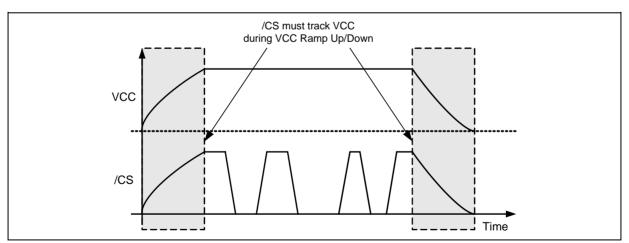
Figure 41b. Power-up, Power-Down Requirement
