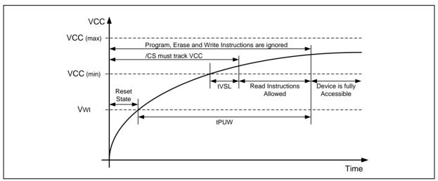
Figure 41a. Power-up Timing and Voltage Levels
