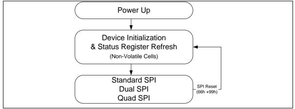
Figure 2. W25Q128JV Serial Flash Memory Operation Diagram
