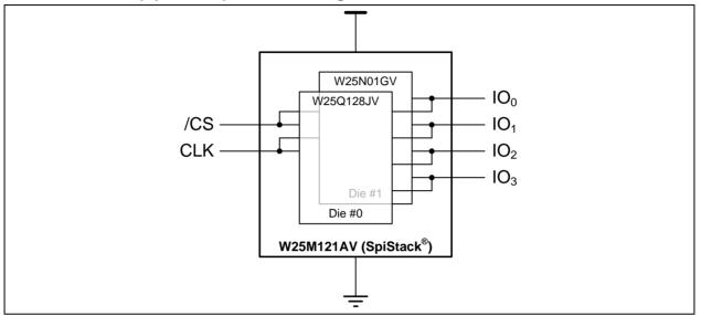
Figure 2. W25M121AV Device Configuration
