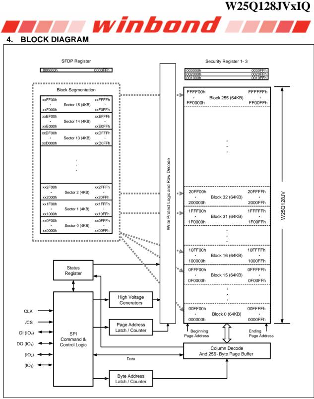
Figure 1. W25Q128JV Serial Flash Memory Block Diagram
