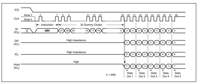
Figure 24b. Fast Read Quad Output Instruction (Continuous Read Mode, BUF=0)
