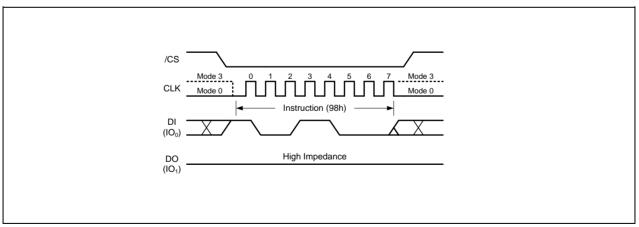
Figure 39. Global Block Unlock Instruction for SPI Mode
