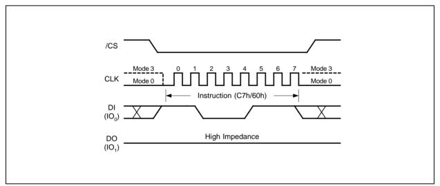
Figure 21. Chip Erase Instruction Sequence Diagram
