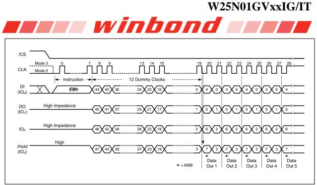
Figure 28b. Fast Read Quad I/O Instruction (Continuous Read Mode, BUF=0)
