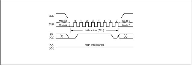
Figure 38. Global Block Lock Instruction for SPI Mode
