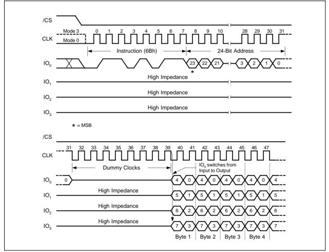
Figure 12. Fast Read Quad Output Instruction
