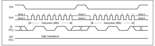
Figure 40. Enable Reset and Reset Instruction Sequence
