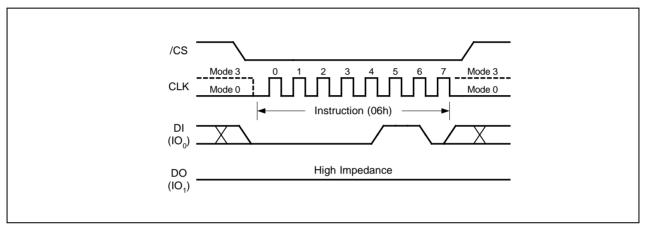
Figure 4. Write Enable Instruction for SPI Mode
