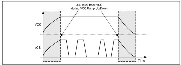
Figure 30b. Power-up, Power-Down Requirement
