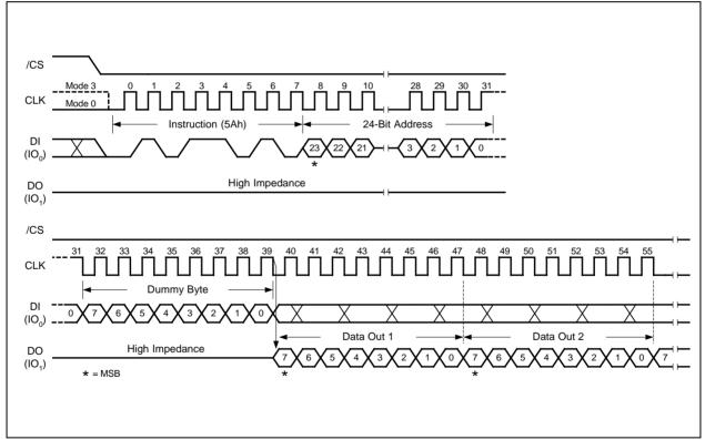
Note 1: A23-A8 = 0; A7-A0 are used to define the starting byte address for the 256-Byte SFDP Register.
