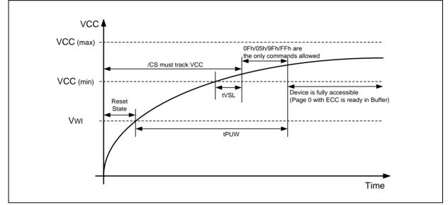
Figure 30a. Power-up Timing and Voltage Levels
