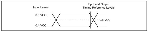
Figure 42. AC Measurement I/O Waveform
