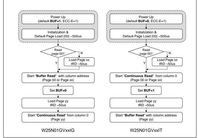
Figure 3. W25N01GV Flash Memory Operation Diagram
