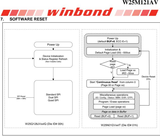
Figure 5. W25M121AV Software Reset Operation Flow
