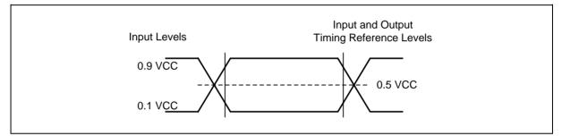
Figure 31. AC Measurement I/O Waveform
