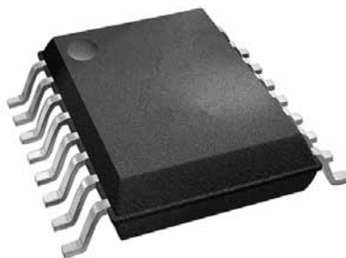
S7 Package 16 Pin Wide Body SOIC with Heat Slug
