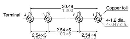
Tolerance:  $\pm 0.1 \pm .004$ General tolerance:  $\pm 0.5 \pm .020$
