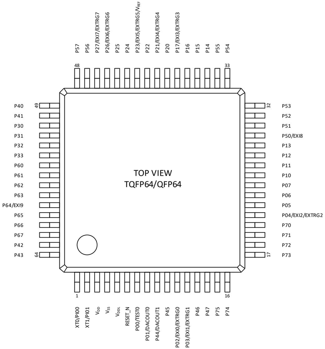
Figure 5 Pin Layout of 64pin TQFP/QFP Package
