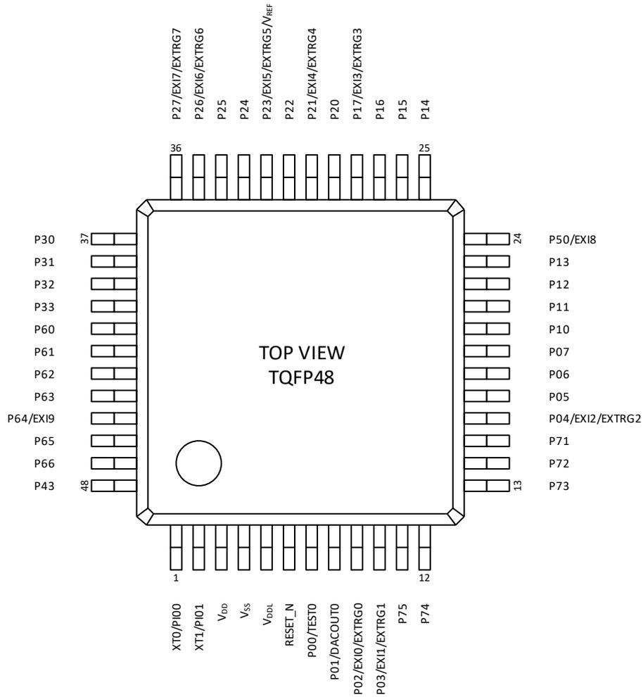
Figure 3 Pin Layout of 48pin TQFP Package
