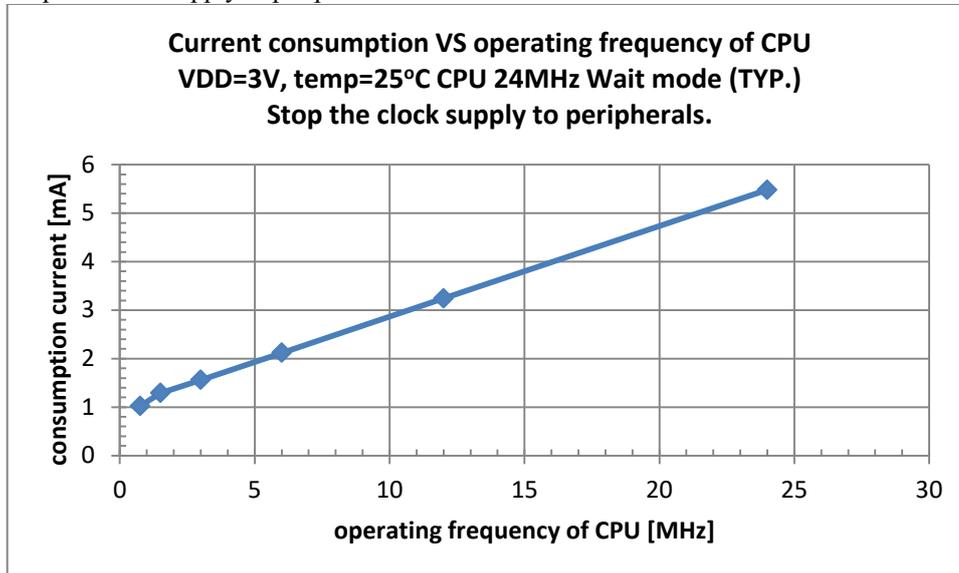
VDD=3V, temp=25°C CPU 24MHz no Wait mode (TYP.)
