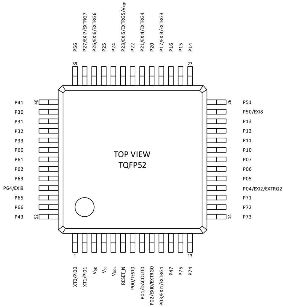
Figure 4 Pin Layout of 52pin TQFP52 Package
