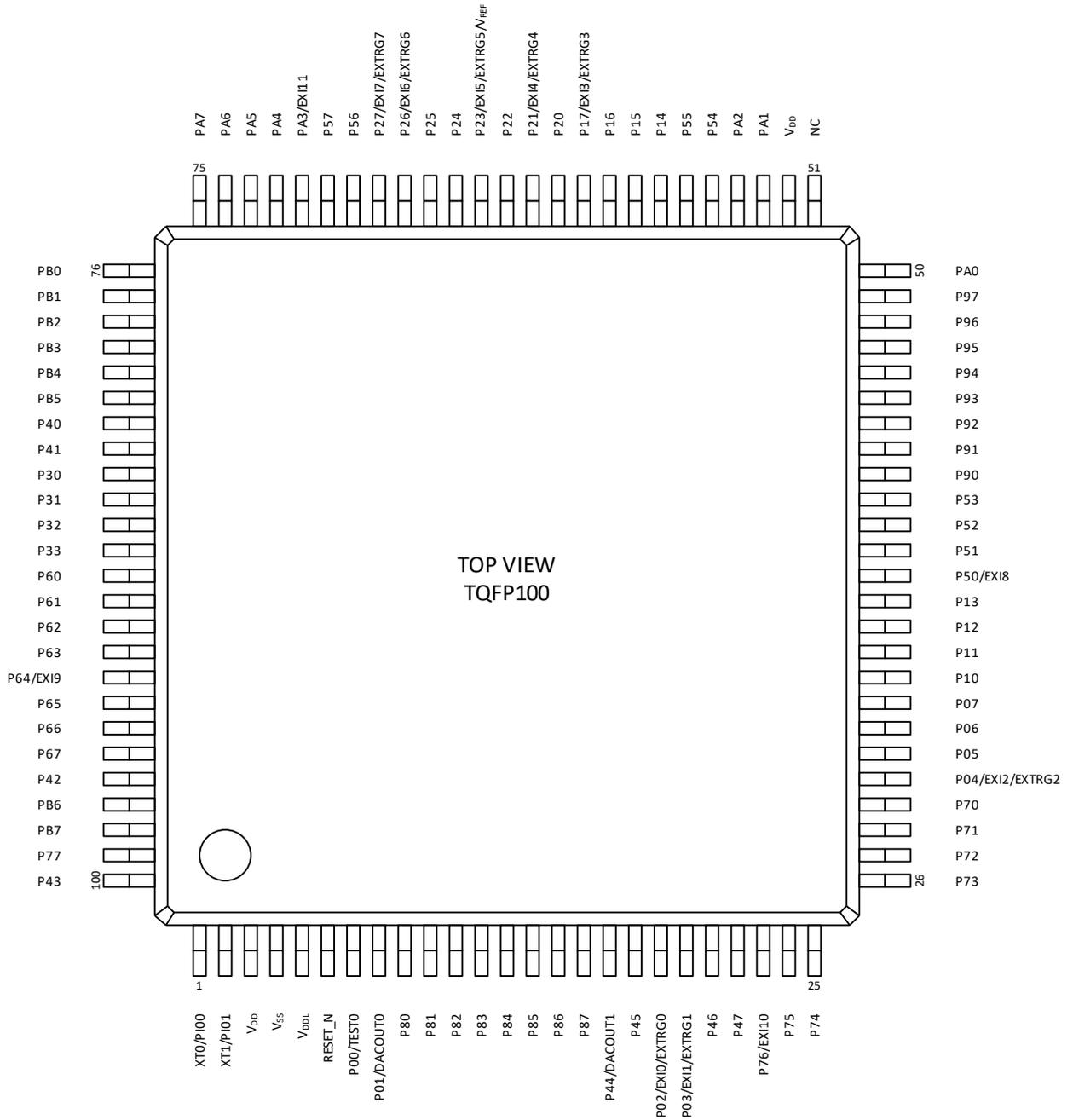
Figure 7 Pin Layout of 100pin TQFP Package
