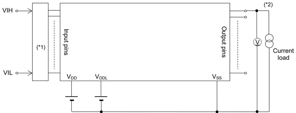
(\*1) Input logic circuit to determine the specified measuring conditions
