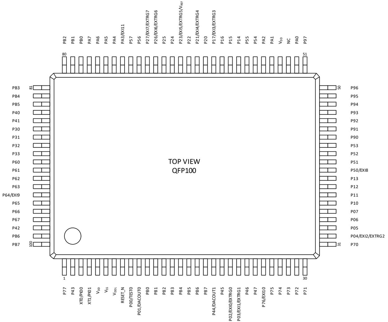
Figure 8 Pin Layout of 100pin QFP Package
