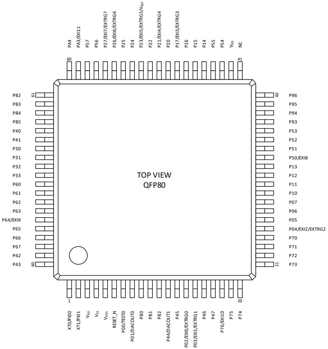
Figure 6 Pin Layout of 80pin QFP Package
