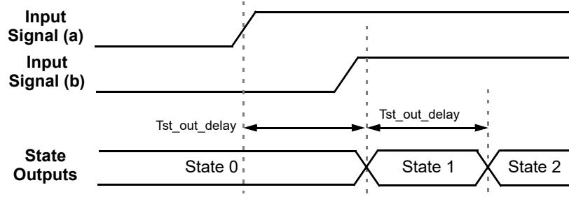
Figure 98. State Transition - Sequential Timing
