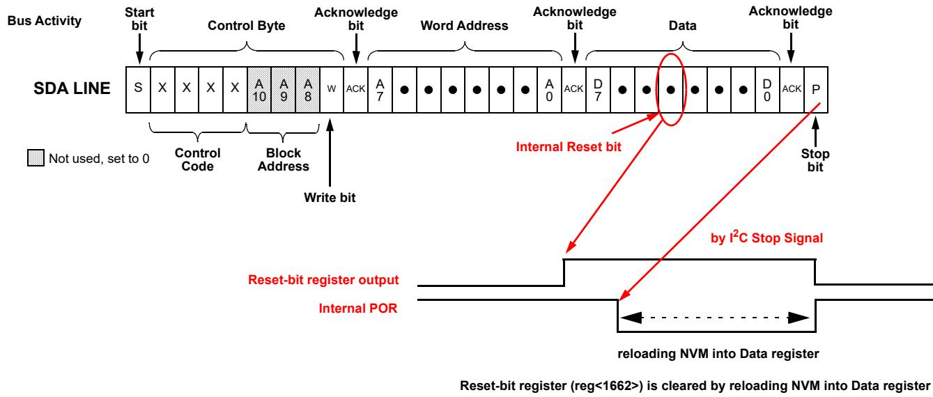
Figure 109. Reset Command Timing
