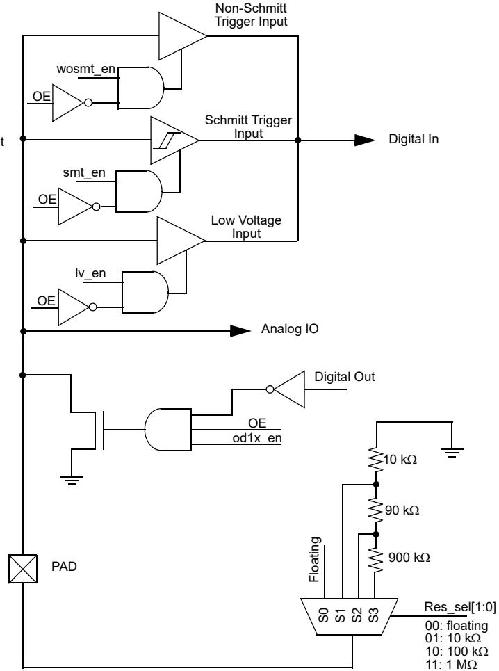
Figure 5. Matrix OE IO Structure Diagram
