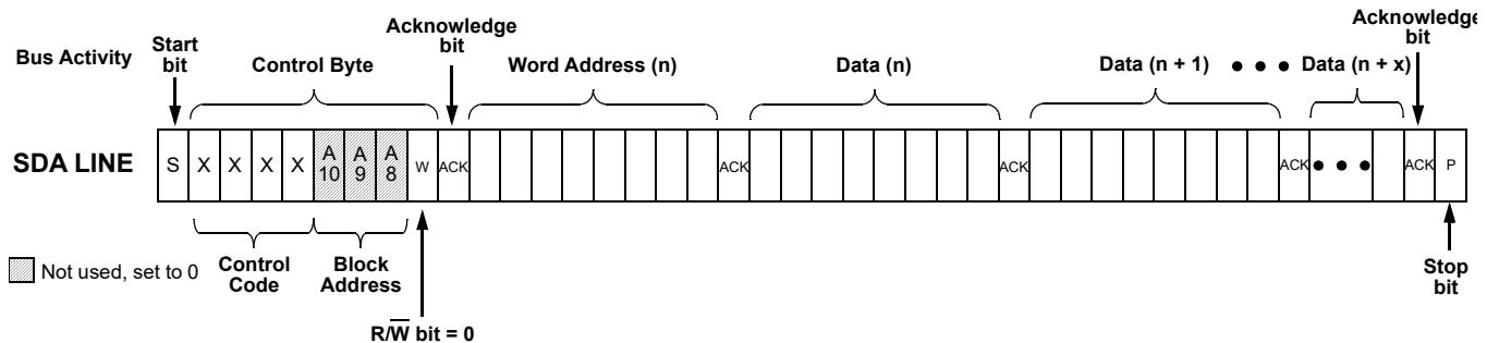
Figure 104. Sequential Write Command,  $\overline{R/W} = 0$
