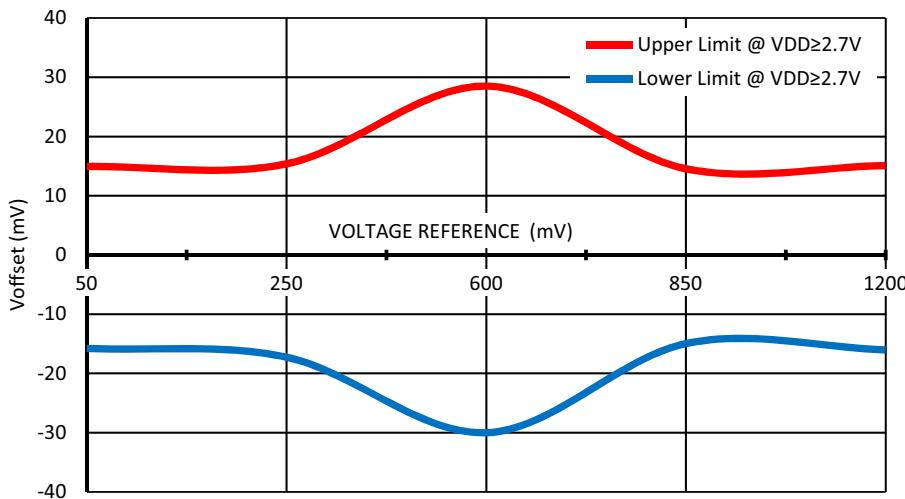
**Figure 54. Typical Buffer Input Voltage Offset vs. Voltage Reference at  $T = (-40 \dots +85)^\circ C$ ,
