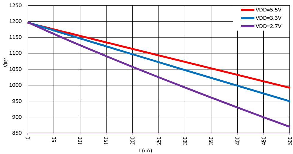
Figure 67. Typical Load Regulation, V<sub>REF</sub> = 1200 mV, T = (-40...+85)°C, Buffer - Enable
