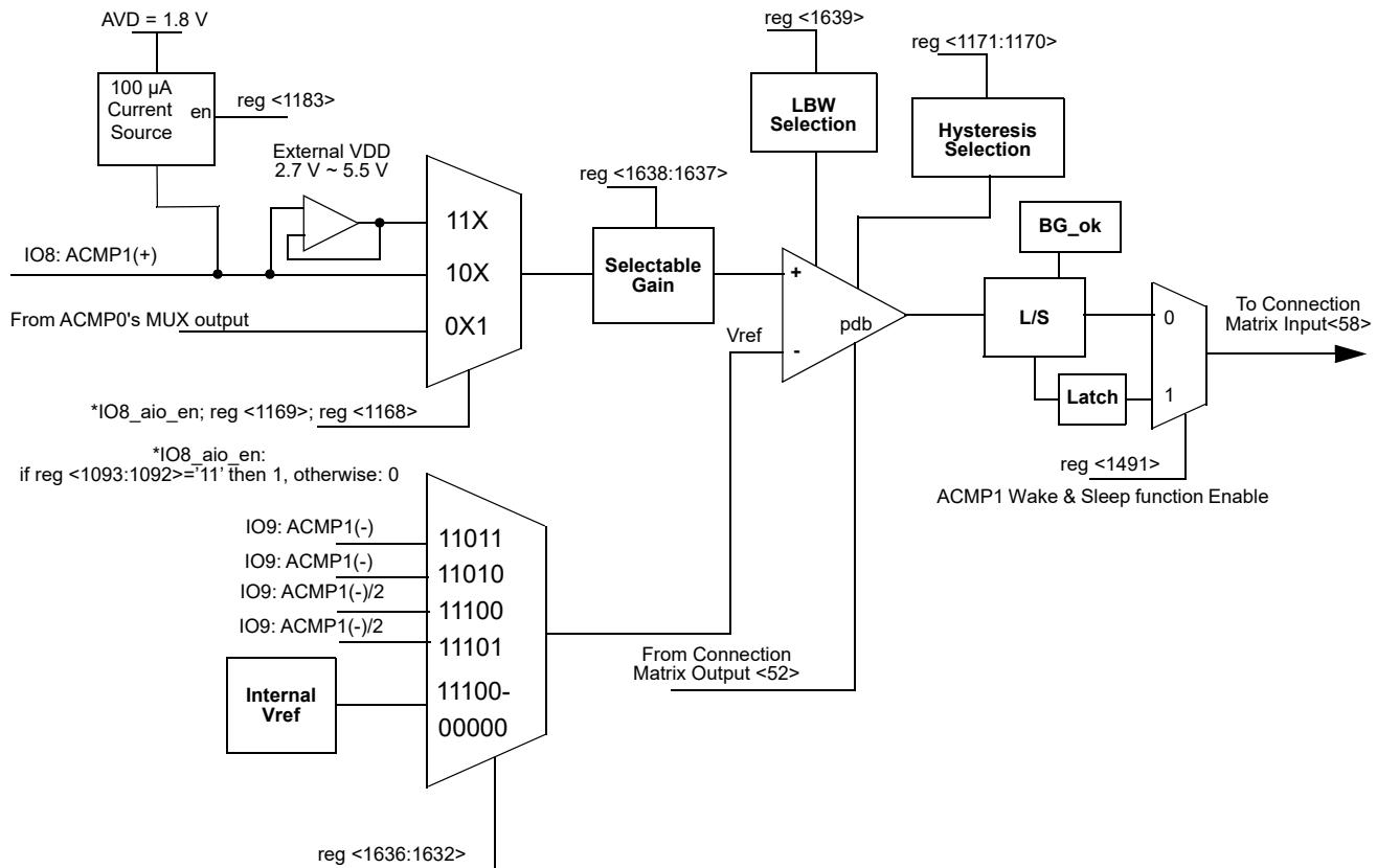
Note: when 100  $\mu$ A Current Source is enabled input voltage on IO8 should not exceed 1.8 V
