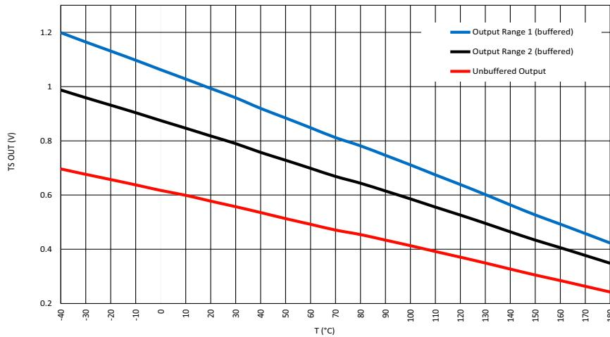
Figure 111. TS Output vs. Temperature, VDD = (1.71...5.5) V
