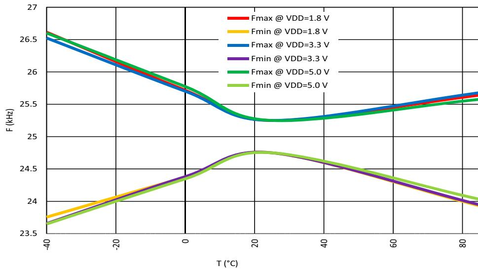
Figure 75. RC Oscillator Frequency vs. Temperature, RC OSC0=25 kHz
