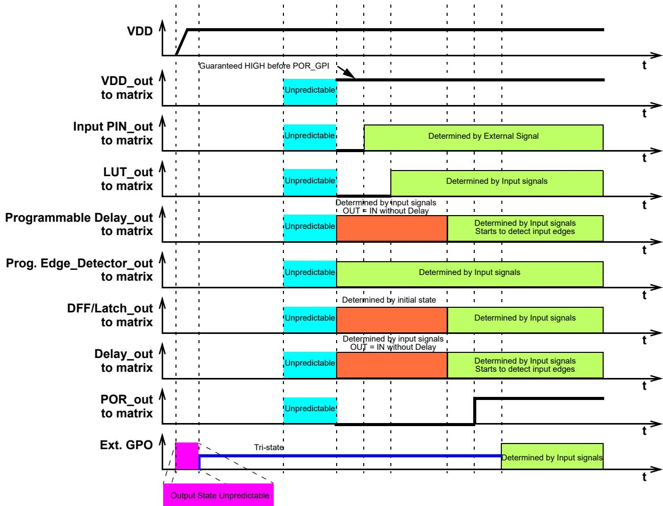
Figure 80. Internal Block States during POR sequence
