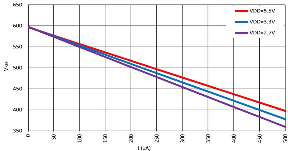
Figure 65. Typical Load Regulation,  $VREF = 600\text{ mV}$ ,  $T = (-40\dots+85)\text{^\circ C}$ , Buffer - Enable
