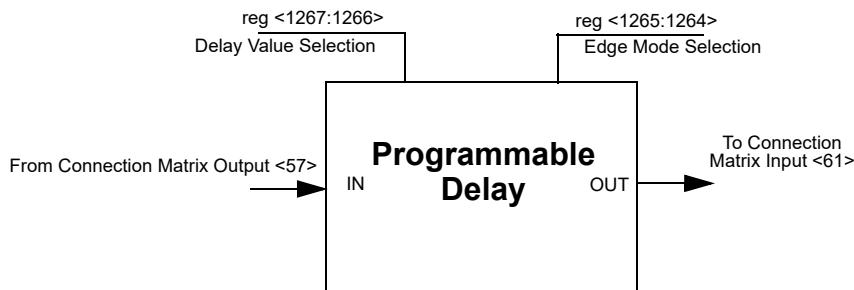
Figure 60. Programmable Delay
