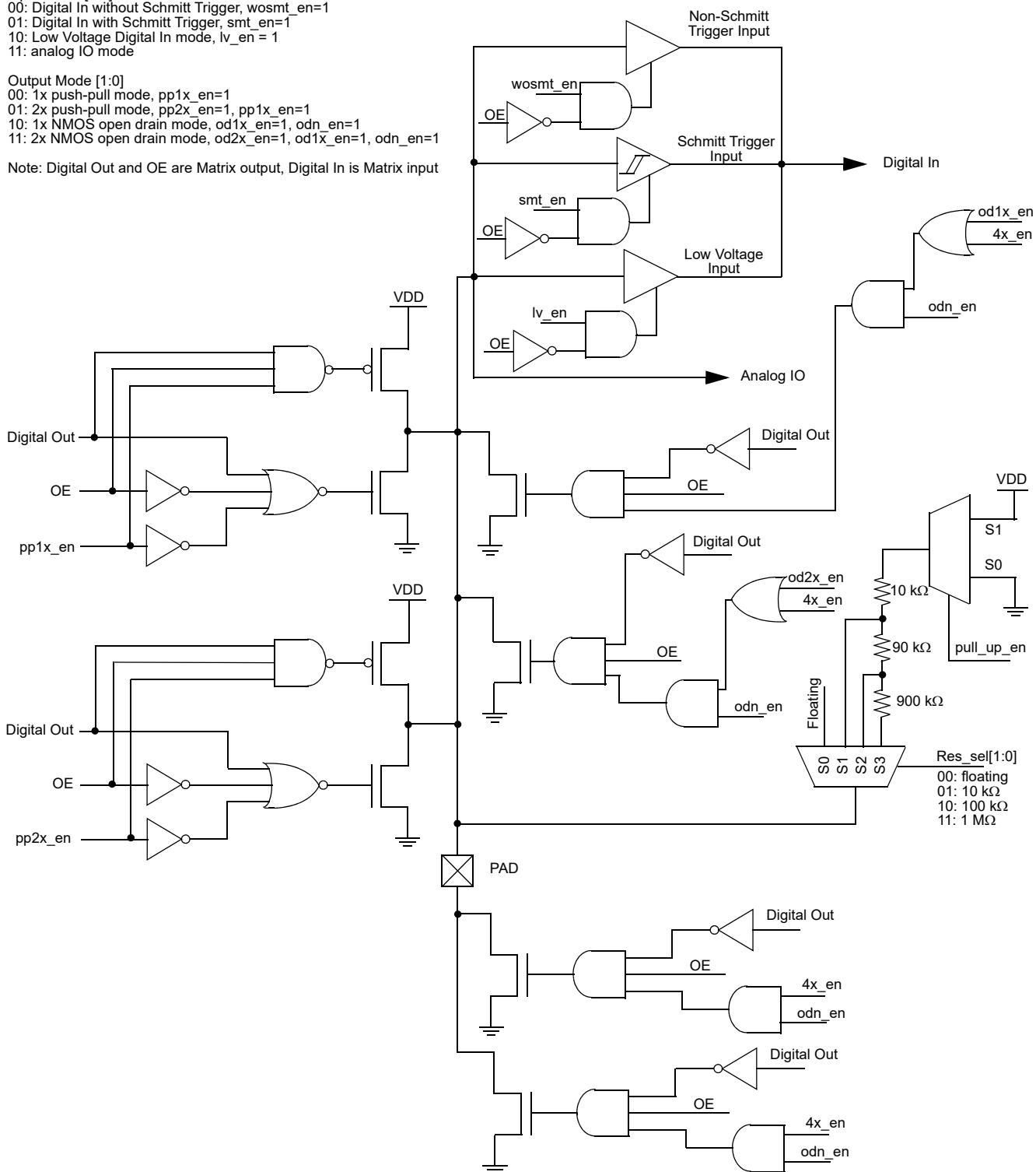
Figure 6. Matrix OE IO 4X Drive Structure Diagram
