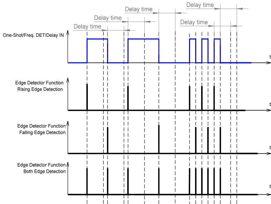
Figure 41. Edge Detection Mode Timing Diagram
