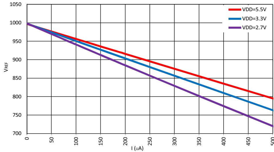
Figure 66. Typical Load Regulation,  $VREF = 1000\text{ mV}$ ,  $T = (-40\dots+85)\text{^\circ C}$ , Buffer - Enable
