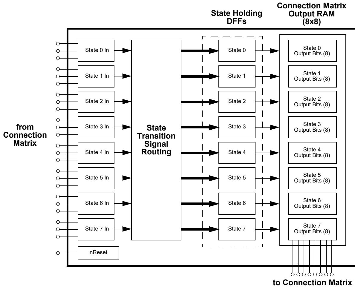
Figure 83. Asynchronous State Machine
