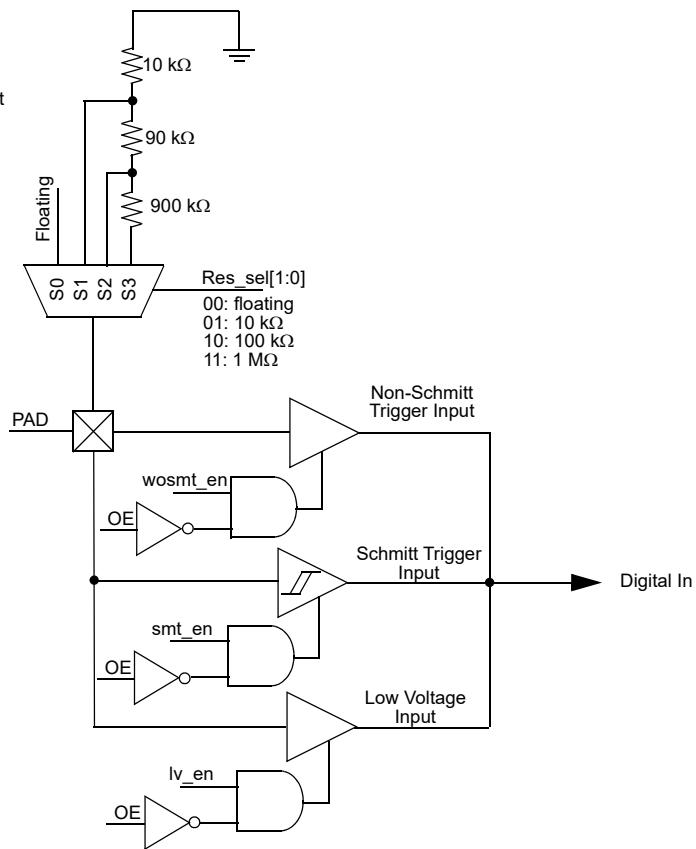
Figure 2. IO0 GPI Structure Diagram
