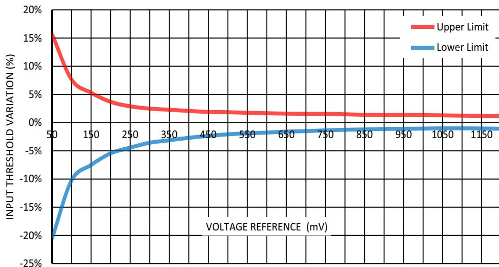
**Figure 55. Typical Input Threshold Variation (including Vref variation, ACMP offset) vs. Voltage Reference at  $T = (-40 \dots +85)^\circ\text{C}$ , LMB Mode - Disable,  $V_{\text{HYS}} = 0 \text{ mV}$ .**
