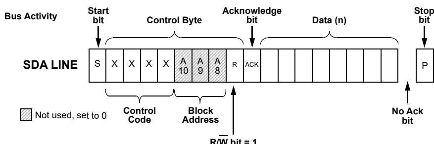
Figure 105. Current Address Read Command,  $\overline{R/W} = 1$
