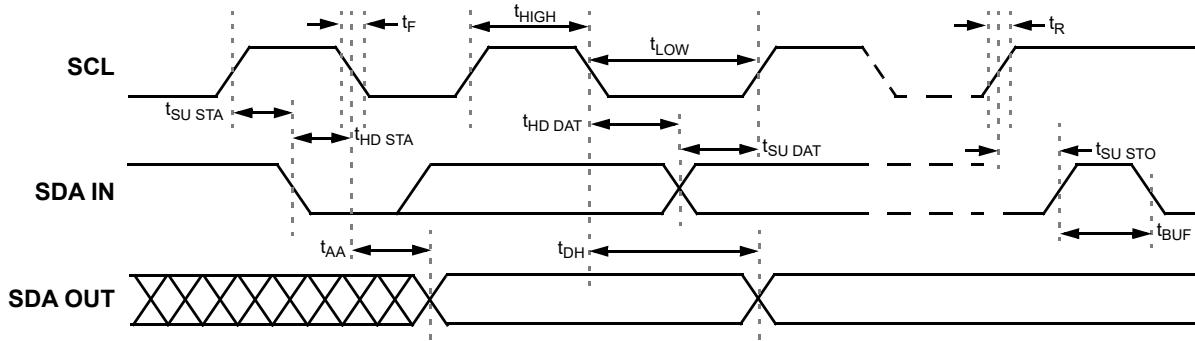
Figure 102. I<sup>2</sup>C General Timing Characteristics
