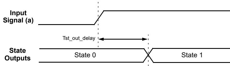
Figure 89. State Transition Timing
