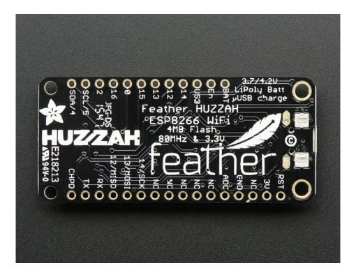
Comes fully assembled and tested, with a USB interface that lets you quickly use it with the Arduino IDE or NodeMCU Lua. (It comes preprogrammed with the Lua interpretter) We also toss in some header so you can solder it in and plug into a solderless breadboard. Lipoly battery and USB cable not included (but we do have lots of options in the shop if you'd like!)
