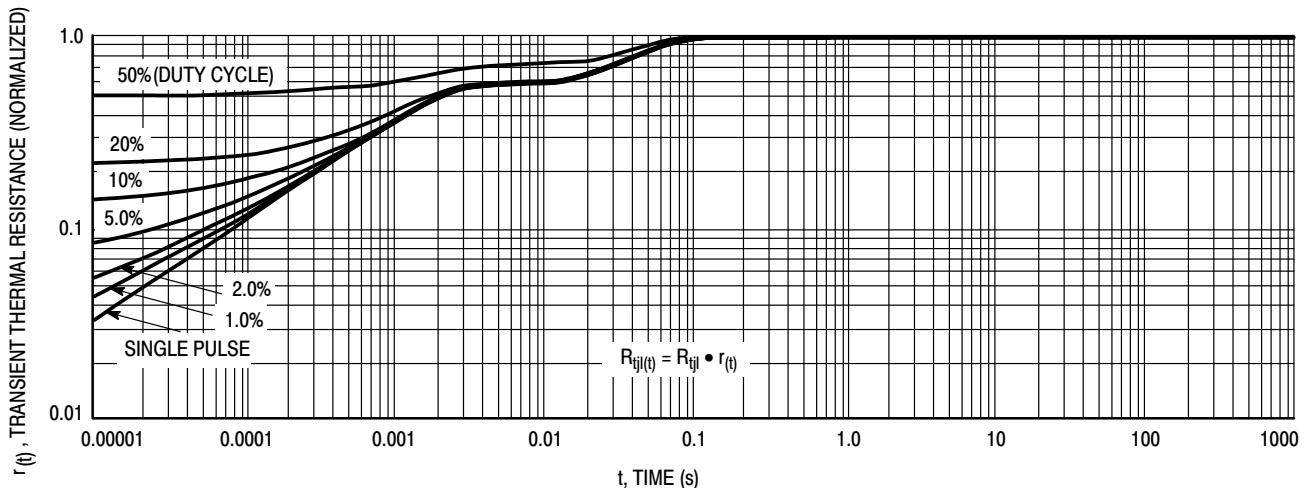
Figure 9. Thermal Response Junction to Case (Per Leg)
