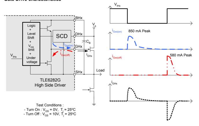
This figure represents the simplified internal circuit of one high side gate drive. The drive circuit of the low sides looks similar.
