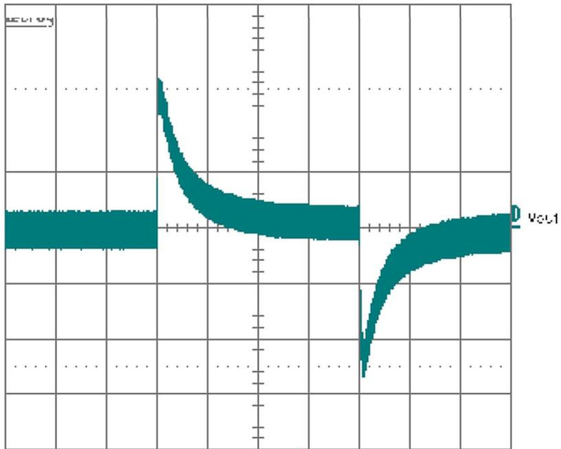
Figure 3. Transient Response, 0A to 35A, 48V<sub>IN</sub> (200mV and 0.5ms/Div)
