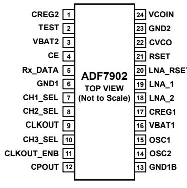
Figure 2. Pin Configuration
