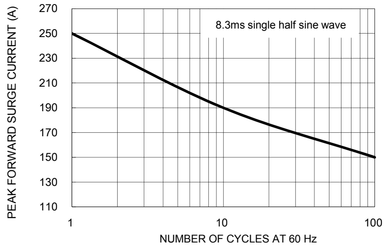
FIG. 7 MAXIMUM NON-REPETITIVE PEAK FORWARD SURGE CURRENT
