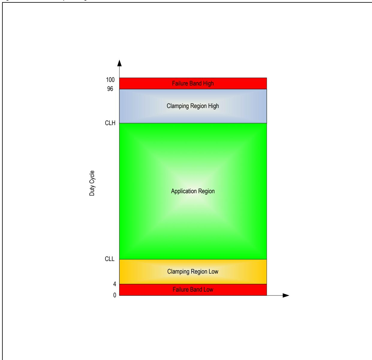
Figure 9 gives an overview about the different ranges. The failure bands are used to indicate a wrong operation of the AS5261. This can be caused due to a broken supply line. By using the specified load resistors the output level will remain in these bands during a fail. It is recommended to set the clamping level **CLL** above the lower failure band and the clamping level **CLH** below the higher failure band.
