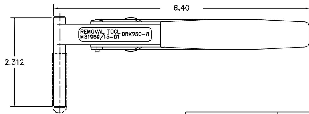
1. WITH TIPS CLOSED AROUND A  $\phi$ .275/.274 PIN, TIPS SHALL ENTER A RING GAGE OF  $\phi$ .318/.317.
