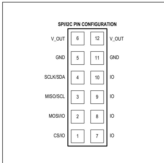
Figure 4. X3: Pmod SPI/I<sup>2</sup>C Connector Pin Configuration
