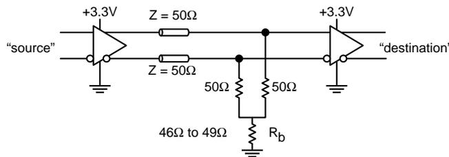
**Figure 2. Three-Resistor "Y-Termination"**
