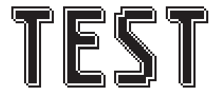
Overlaying (EXOR) of the "outline font" at pos. 2,2. results in an "outline font with fill"
