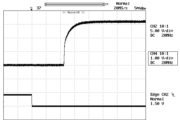
Figure 4: (For negative remote on/off logic) Turn-on transient at full rated load current (5 ms/div). Vin=48V. Top Trace: Vout, 1V/div; Bottom Trace: ON/OFF input, 5V/div.
