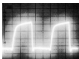
Signal Waveform (20ns/div / 1V/div)
