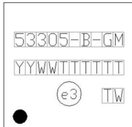
Figure 8.6. Si53305 Top Marking
