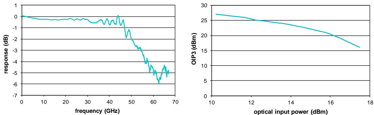
Fig. 1: Frequency response measured with a Lightwave Component Analyzer.
