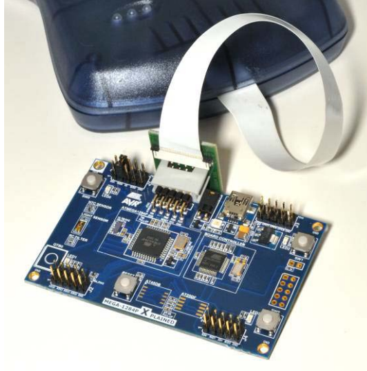
Figure 4-2. Connecting AVR JTAGICE mkII to an Xplained board.
