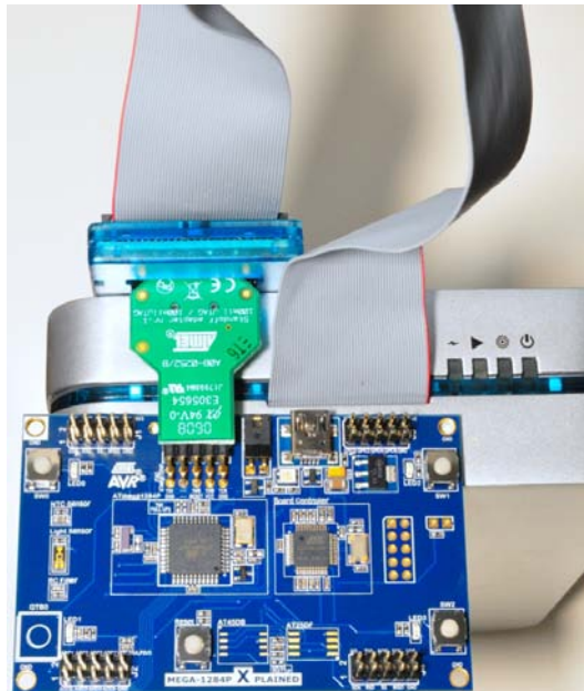
Figure 4-3. Connecting AVR ONE! to a Xplained board.
