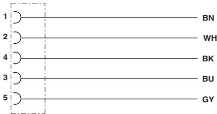
Contact assignment of the M12 socket
