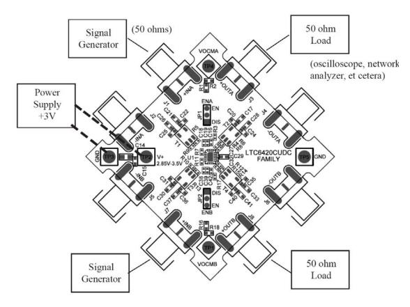
Figure 1: Proper Measurement Equipment Setup
