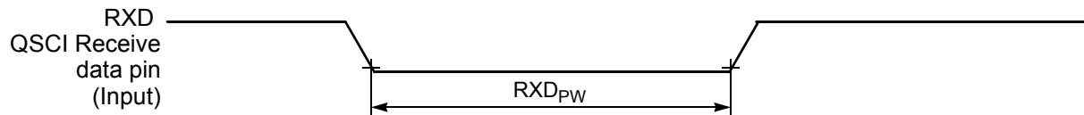
Figure 10-12 RXD Pulse Width
