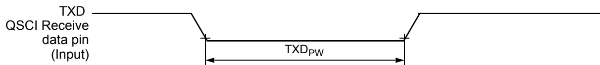
Figure 10-13 TXD Pulse Width
