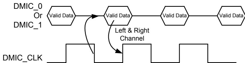
Figure 6. Stereo Digital Microphone Configuration
