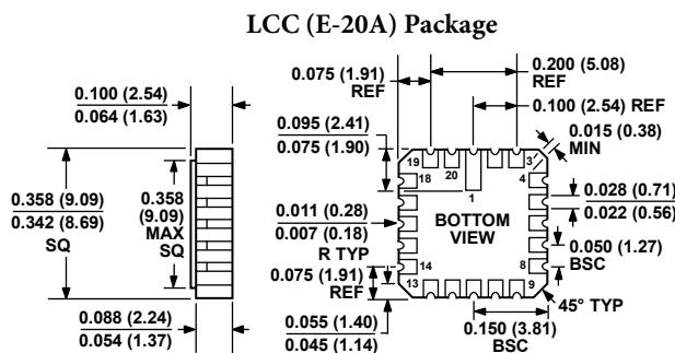
CONTROLLING DIMENSIONS ARE IN INCHES; MILLIMETER DIMENSIONS
