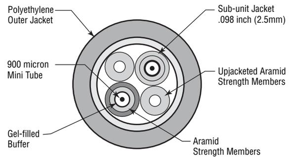
**Micro Loose Tube Breakout Style Cable**Loose Tube – Outdoor, Indoor/Outdoor OFN & Indoor/Outdoor Riser Rated (*continued*)
