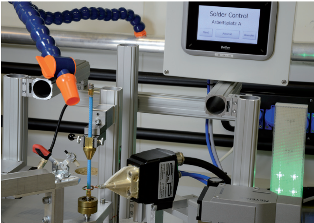
Temperature controlled soldering
