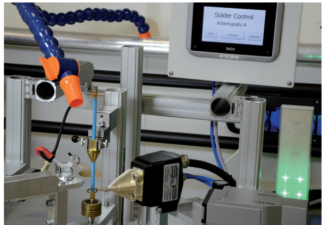
Temperature controlled soldering
