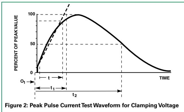
**Figure 2: Peak Pulse Current Test Waveform for Clamping Voltage**
