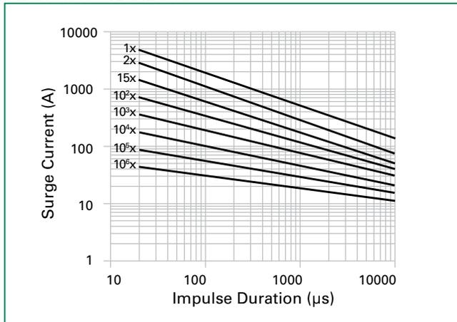
NOTE: If pulse ratings are exceeded, a shift of  $V_{NIDCI}$  (at specified current) of more than +/-10% could result. This type of shift, which normally results in a decrease of  $V_{NIDCI}$ , may result in the device not meeting the original published specifications, but does not prevent the device from continuing to function, and to provide ample protection.
