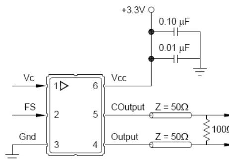
**LVDS to LVDS:** The 100Ω resistor should be removed if this load is provided internally within the LVDS receiver.
