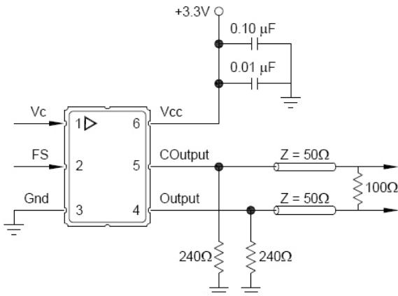
**LV-PECL to LV-PECL:** For short transmission lengths, the pull down resistor values shown provide reasonable power consumption and waveform performance.
