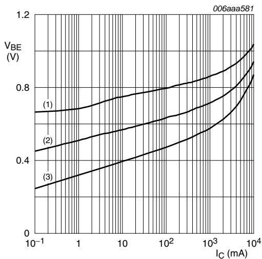
**Fig 7.** Base-emitter voltage as a function of collector current; typical values
