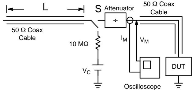
Figure 13. Simplified Schematic of a Typical TLP System
