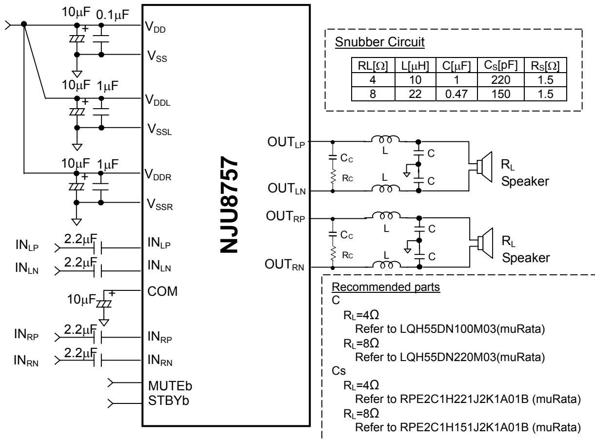
Figure3. Application Circuit example
