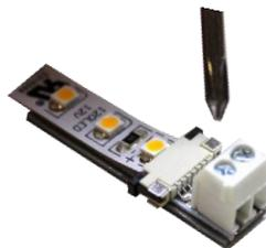
**7** Strip cable back ¼" to expose (+) and (-) wire, (if using Inspired LED cable, white writing indicates positive polarity)
